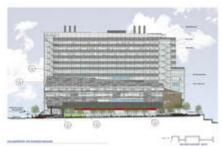
The south elevation shows the "south bar" in relation to the "north tower." The band of darker grey above the red is a perforated metal "skirt" that provides sun screening in the summer months to the large expanse of glazing at the retail area on the ground floor. - Photo Credit: SERA Architects
