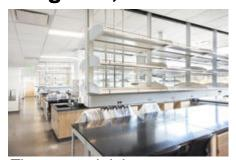
The research lab areas are laid out in open modules to allow for flexibility in usage by different researchers with differently scaled projects over time. The bench layout is perpendicular to the exterior windows to maximize daylighting penetration.
