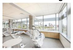
Recognizing the importance of natural light and its link to productivity and health, the design team strove to daylight all regularly occupied spaces, while mitigating heat gain, by providing filtered light through shades attached to window mullions located above the view area. - Photo Credit: Alene Davis Photography
