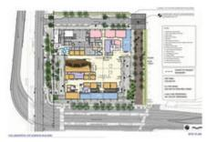
The first floor of the building is designed to integrate with the site, allowing pedestrians views deep into the building. The ground floor of the atrium connects directly onto outdoor plazas on the east and west. Hearty, native plantings were used throughout and serve as part of the stormwater management system. - Photo Credit: SERA Architects & Mayer/Reed
